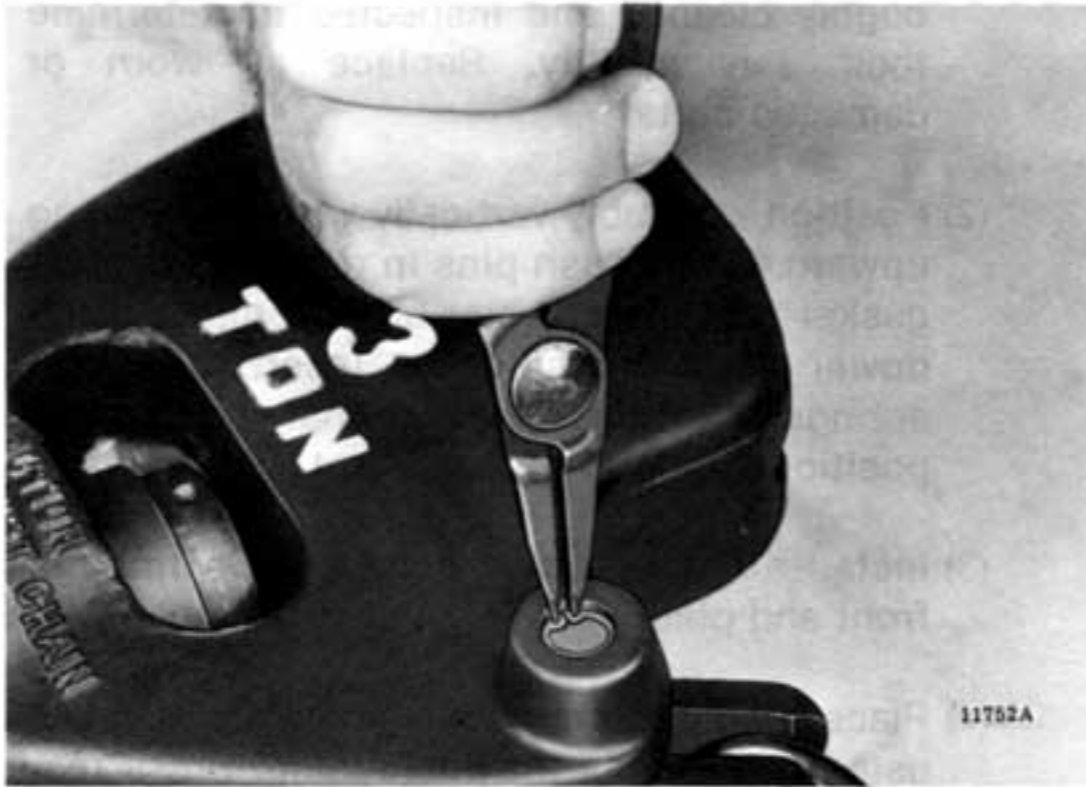
Figure 7-27. Removing Retaining Ring From Bore of Connecting Link Pin — Triple Reeved Lower Block Assembly.
